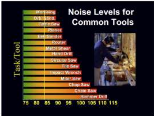
Fig. 1—Tools and tasks vs. Noise level demonstrate carpenters' noise exposure 8 . Sound pressure level in A-weighted dB measured at typical operator's ear distance.
